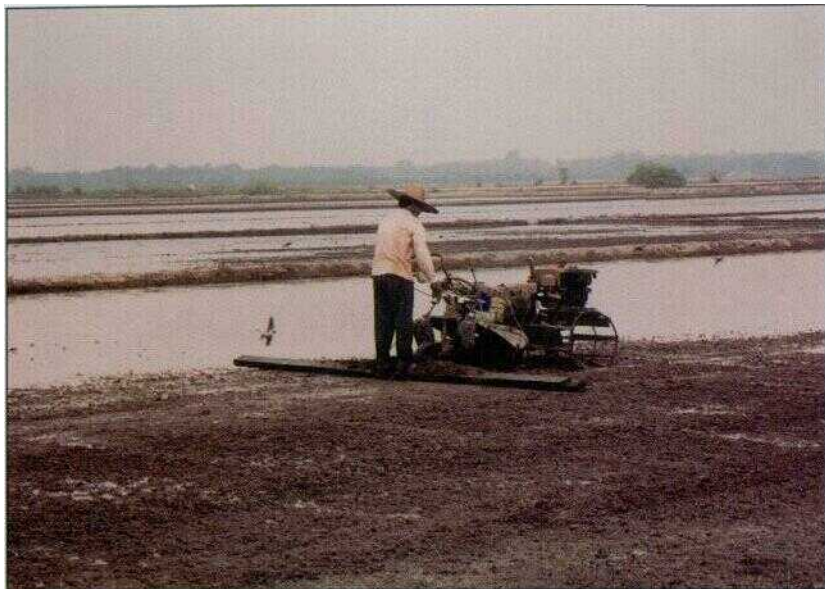
Use of a pedestrian tractor for in-field soil surface smoothing
